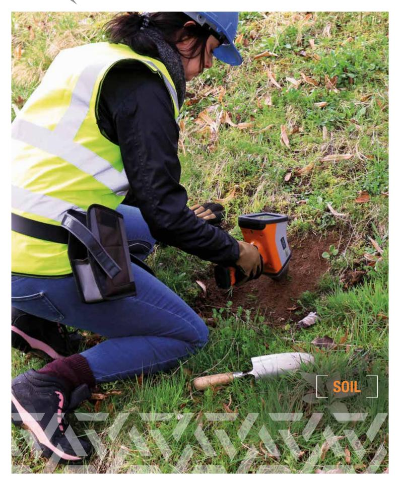
The X-MET8000 Expert Geo is an X-ray fluorescence (XRF) analyser for on-site environmental soil and sediment screening. Carry out high volumes of analyses and complete testing programs quickly, reducing the need for laboratory analyses and their associated costs.
